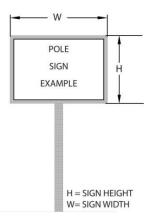
c. **Sign Height**: Height shall be the distance from the top of the sign structure to the lowest grade level of the base of the sign. The height of any monument base or other structure erected to support or ornament the sign shall be measured as a part of the sign height.
