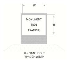
b. **Sign Area, Pole**: The sign area shall be measured as the area enclosed by the smallest single rectangle that will enclose the structure exclusive of the poles.
