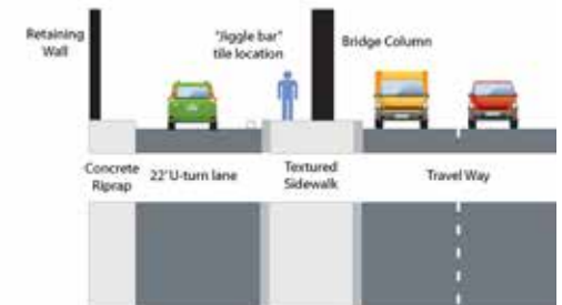
Bridge Redevelopment Possibilities: Reconstruct Retaining Wall Move U-turn lane Enhanced Lighting Column Artwork
