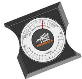
The slope can be determined by standing on the ground, sighting along the top edge of the angle and pitch locator and reading the slope in inches of rise per 12 inches of run. The device can also be placed directly on the roof slope and read there.
