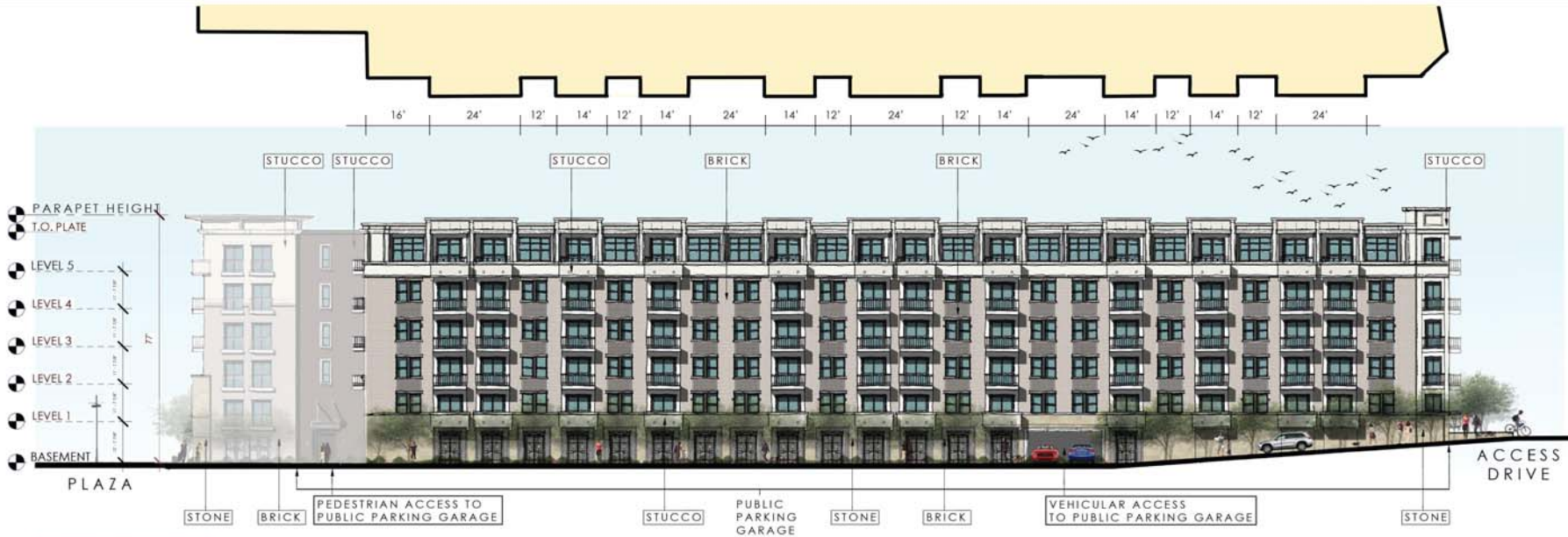
1 BUILDING - WEST ELEVATION SCALE: 1/16" = 1'-0"
