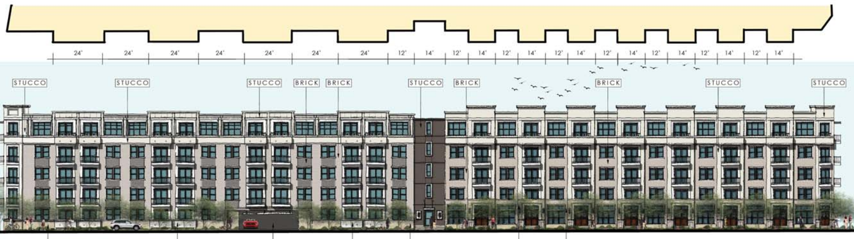
2 BUILDING - SOUTH ELEVATION SCALE: 1/16" = 1'-0"
