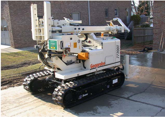
This drilling rig is 8 ft wide and would be a typical drilling rig used in a residential geothermal installation.
