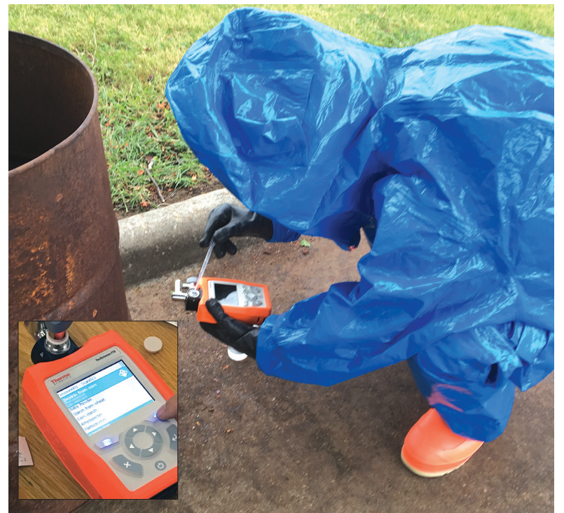
A Richardson firefighter practices using a "TruDefender" tool, a handheld spectrometer that can help first responders identify unknown substances in the field. The tool was purchased with a federal grant through the Homeland Security Grant Program.
