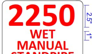
Street Address Number With Wet [or Dry] Auto- matic [or Manual] Standpipe(S)
