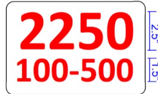
Street Address Number With Unit Range When System Protects Part of Building
