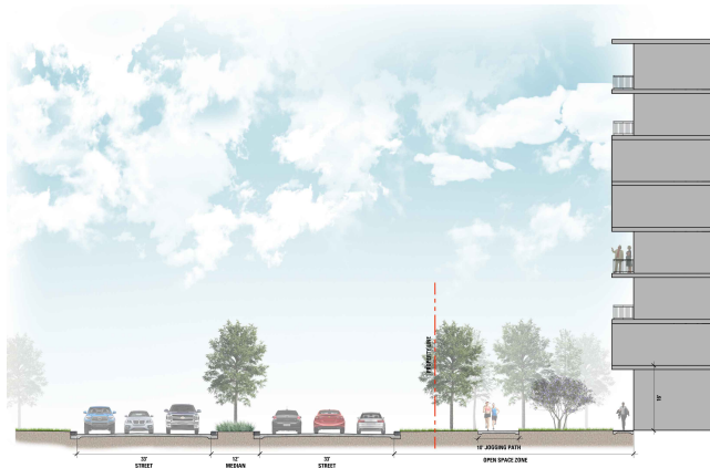
OPEN SPACE & TRAIL SECTION ALONG WATERPARKWAY, TYP. SCALE: 1/4" = 1'-0"
