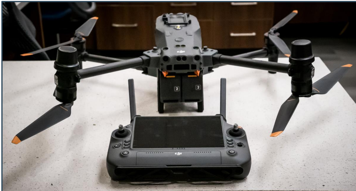
DJI M30T with thermal capabilities and digital zoom of 200X
