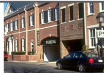
+ PARKING STRUCTURE FENESTRATION Entrances to parking garages should be incorporated into the building facade to provide a seamless frontage along the street.
